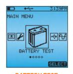
BATTERY TEST Standard, conductancebased battery testing.
